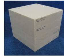
Figure 3. The phantom consisted of four pieces of water equivalent material.
