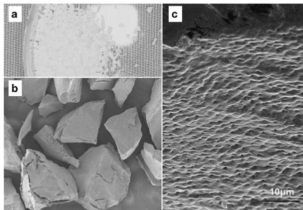
Fig. 3. Aspects of DDM granules. a. freeze-dried DDM before graft, b. SEM of DDM, c. higher magnification of b. Note: Dentinal tubes.
