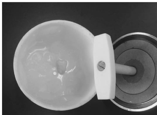
Fig. 1. Extracted tooth with 20 ices in ZrO<sub>2</sub> vessel before crushing.
