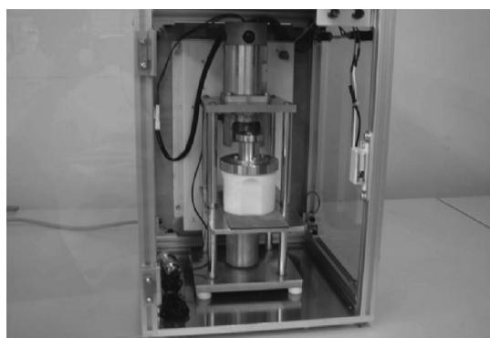
Fig. 2. Automatic mill. Newly developed mill (Patents: International application No. PCT/JP2007/053321, International published No. WO2007/099861 A1).
